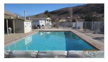
Pool - Deck Caulking, Deco-Seal, Repl. We have budgeted for this every 8 years beginning in 2021. Expansion joints should be replaced at this point. Per information from Lynn the drain needs new grates also.
